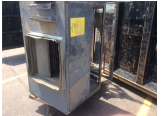
An old Air Handling Unit past its useful life will be replaced with new energy efficient equipment improving indoor air quality.
